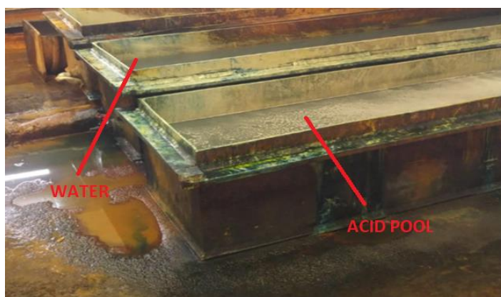
Figure 1. Acid pool and clean water pool
