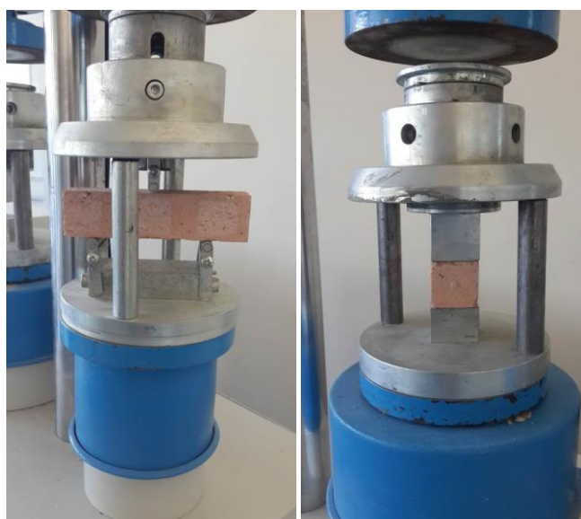
Fig. 10 and 11. Flexural and compressive strength tests.
