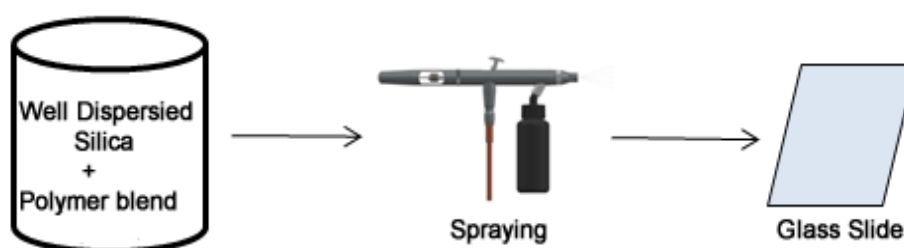
Figure 1. The schematic illustration of spray coating process
